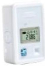
**HIM** : 1 RGB LED + 1 touch-sensitive button + 1 LCD display**Communication** : LoRa® 868MHz or 915MHz\***Memory** : 10 000 time-stamped measurements**Sensor** : Inside control unit**Operating range** : -30+70°C**Measurement range** : -30+70°C and 0 – 100% RH**Accuracy, standard version****Temperature** : ± 0.4°C from -20 C° to +40°C / ± 0.5°C outside this range**Humidity at T° between 15 and 25°C** : ±2% HR from 20% to 80%
