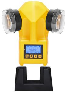
The Stand up fixed on the surface of the cart guarantees the stability of the instrument during movements. It also makes the instrument independent from the cart
