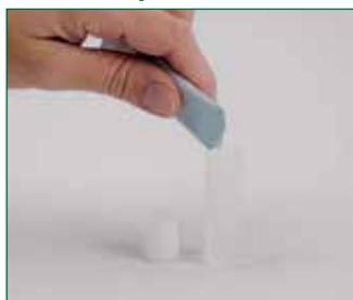
1. Open Type 11 extraction buffer sachet and add to a sample tube.
