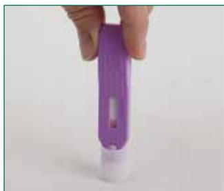
3. Leave the cavity saturated until the liquid is seen running into the test window.
