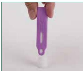
2. Dip the Reveal device into the liquid in the lid; ensure that the cavity is saturated with the liquid.
