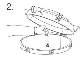
Place one capsule (or 2 if the odor is strong) in the water at the bottom of the autoclave.
