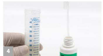
4 Add 800 µL of sample extract into a new Reveal 3-D for Gluten Extraction Buffer bottle. Cap and invert to mix. Proceed to Sample Testing.
