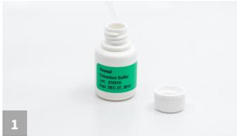
1 Add 0.25 mL of sample into an extraction buffer bottle.
