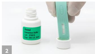
2 Dip the device into the lid, and leave in until liquid is in the test window.
