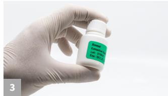
3 Secure cap and shake for 1 minute. Proceed to Sample Testing.
