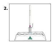
Take one AgraStrip® Total Milk test strip from its container and place it vertically (sample pad downwards) into the incubation vial. Incubate for **5 minutes**.
