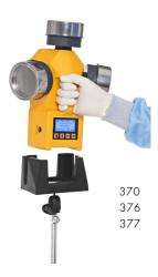
The stand up fixed on vertical support lets the air sampler independent from the cart. The operator is facilitated when he has to remove the instrument to charge the batteries and the Petri dishes after sampling.
